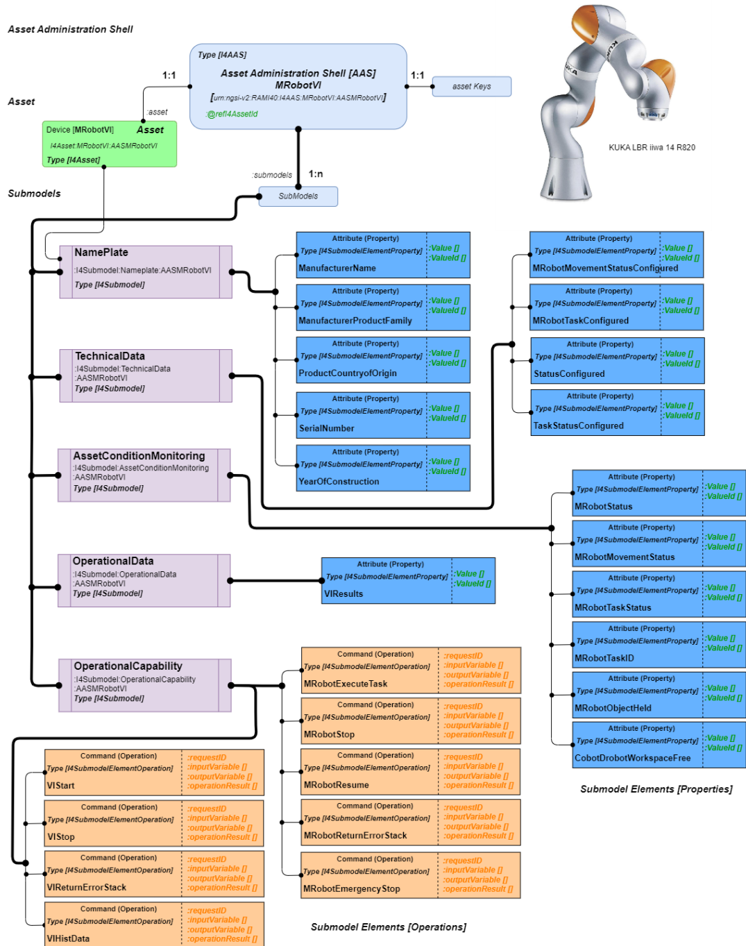
Figure 4. Example of the Digital Twin structure defined within CoRoSect. Represents the MRobotVI DT.
