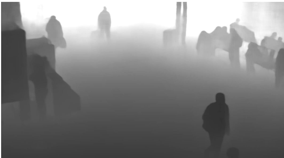
Figure 5 - Depth map example using CV from a monocular camera
