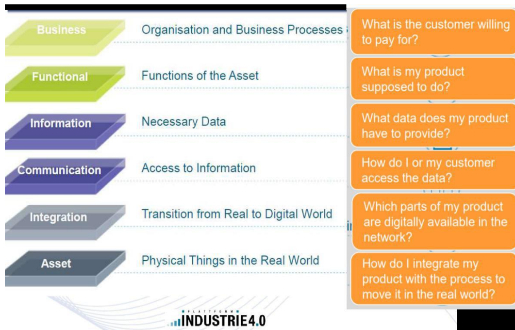
Figure 37. Vertical Axis of RAMI 4.0 and its descriptions [24]
