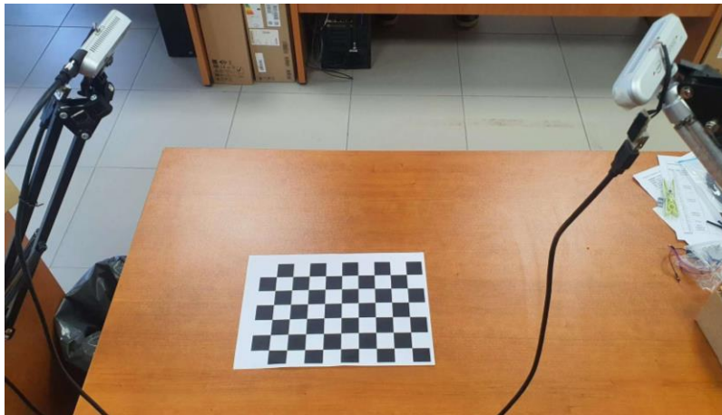
Figure 4. Camera Setup to capture hand and object for both angles
