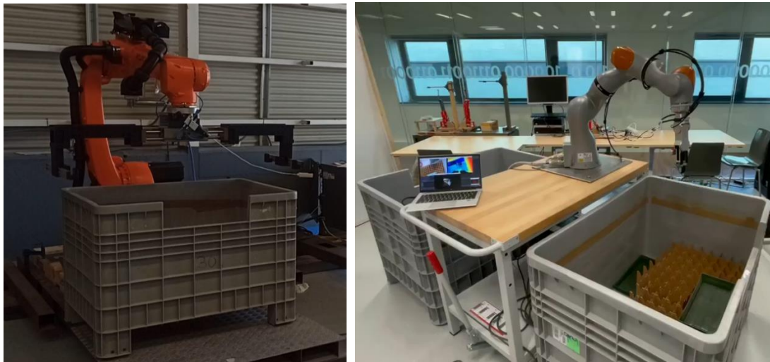
Figure 6: (left) Robot for handling crates. Here a crate for rearing crickets is shown. (right) Robot for handling insects. Here the robot is shown handling material for insect rearing inside a crate.
