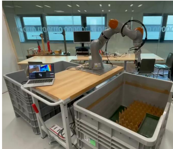
Figure 13. Robot cell for handling insects (M-robot). Left: KUKA LBR iiwa robot arm with extension and gripper picking a drinking device for insects from a crate. Right: KUKA LBR iiwa robot arm with extension and gripper handling material on a pallet.
