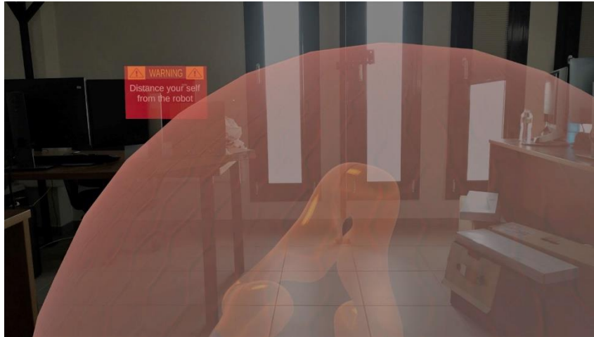
Figure 19. Red 3D Safety-Sphere and warning message is provided when the human co-worker is getting too close to the movement range of the robot
